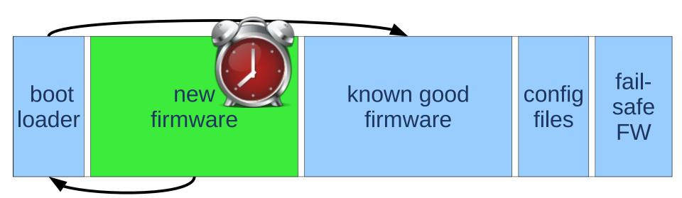
Reboot when watchdog timer expires Reset watchdog if firmware runs well Force reboot if firmware does not run well
